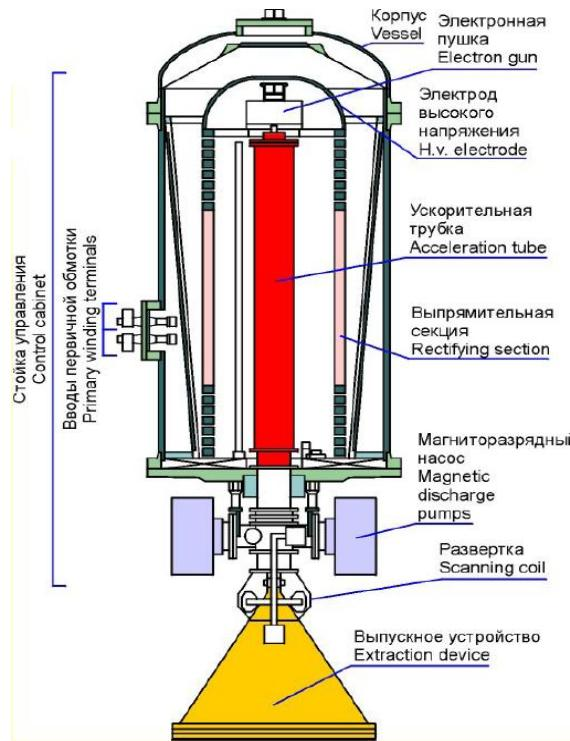
The electron beam power of ELV-12 can reach 400kW with electron energy of 0.6-0.9MeV, and the electron energy of ELV-8 can be 1.0-2.5MeV with beam power of 90kW .
