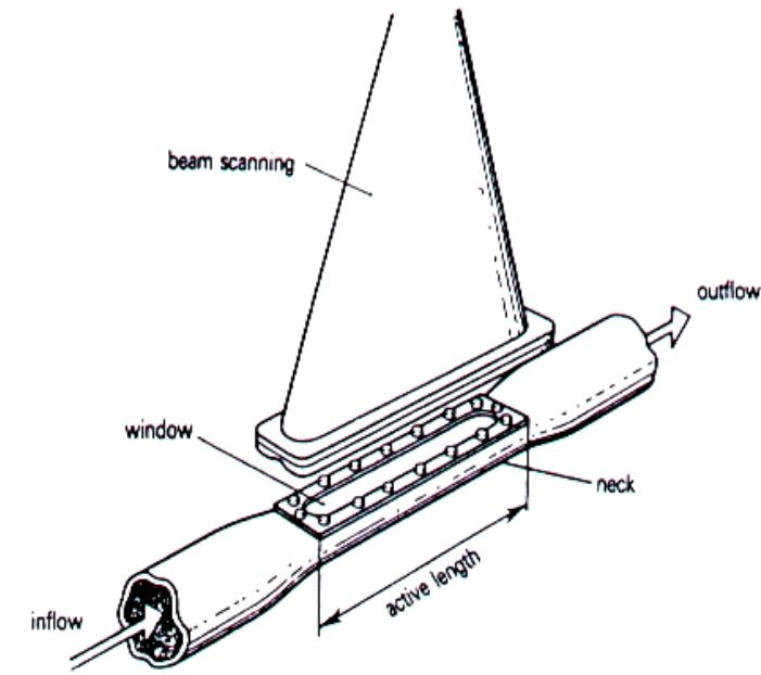
Figure 2.6 (a) Two-sided irradiation of thin foil
