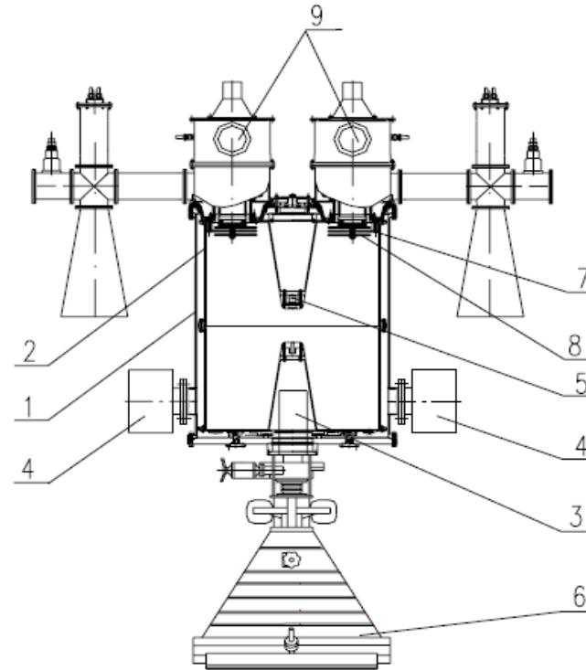
ILU covers the energy range from 0.6MeV to 5 MeV, and the maximum beam power is 50 kW. A 5MeV/300kW ILU accelerator is developing now.
