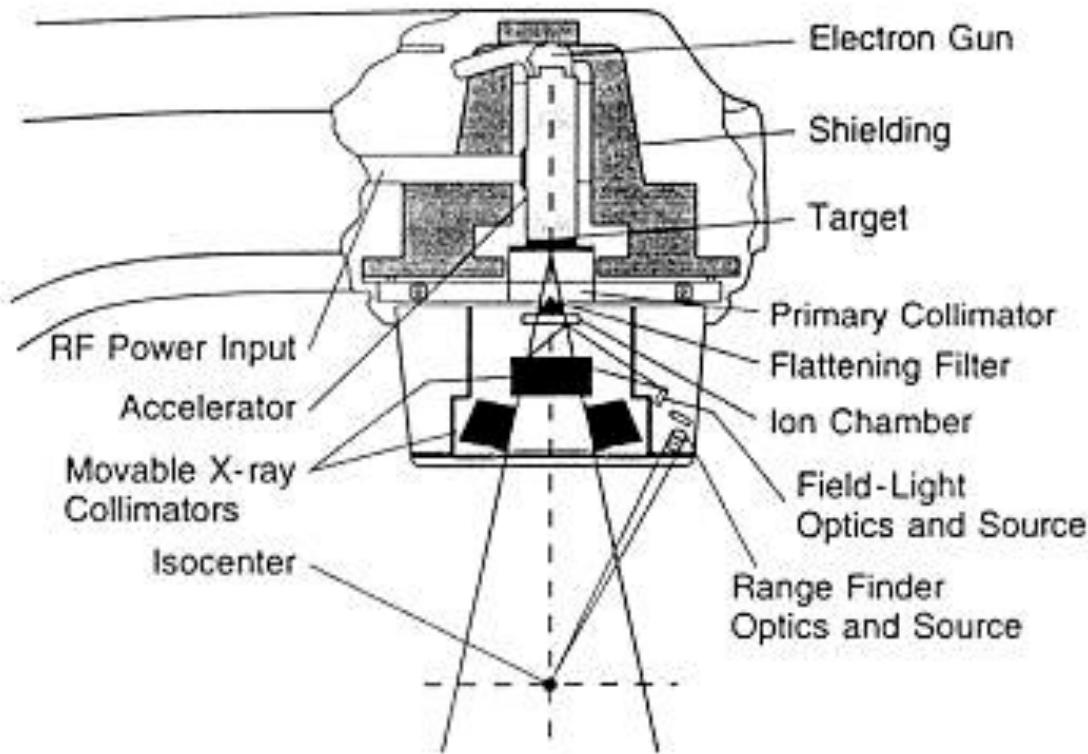
**Figure 1.20 Schematic of a treatment head of Varian clinac 6/100 accelerator for X-ray therapy**
