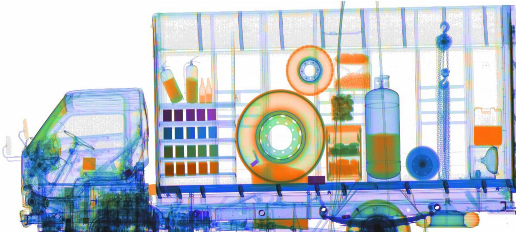
Dual-Energy Color Image: obtained by processing of dual-energy material discrimination algorithm according to effective atomic number
