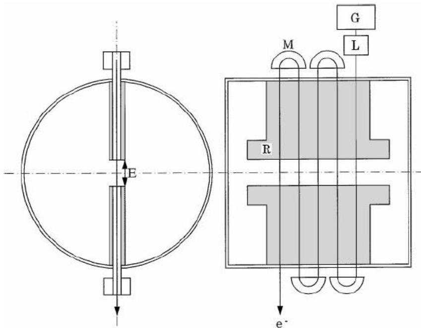
Fig. 1. The schematic drawing of the Ridgetron prototype. G: electron gun; L: solenoid lens; M: deflector magnet; R: hollow ridge; E: electric field.
