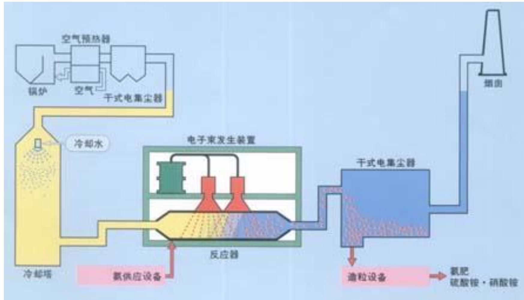
Figure 2.4 The principle of EFGT's technique
